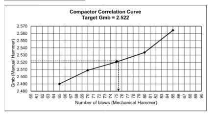
Based on the correlation chart, the laboratory will use 75 blows per face.
